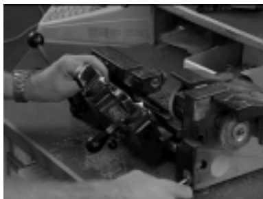
Use key-cutting machine to duplicate keys
